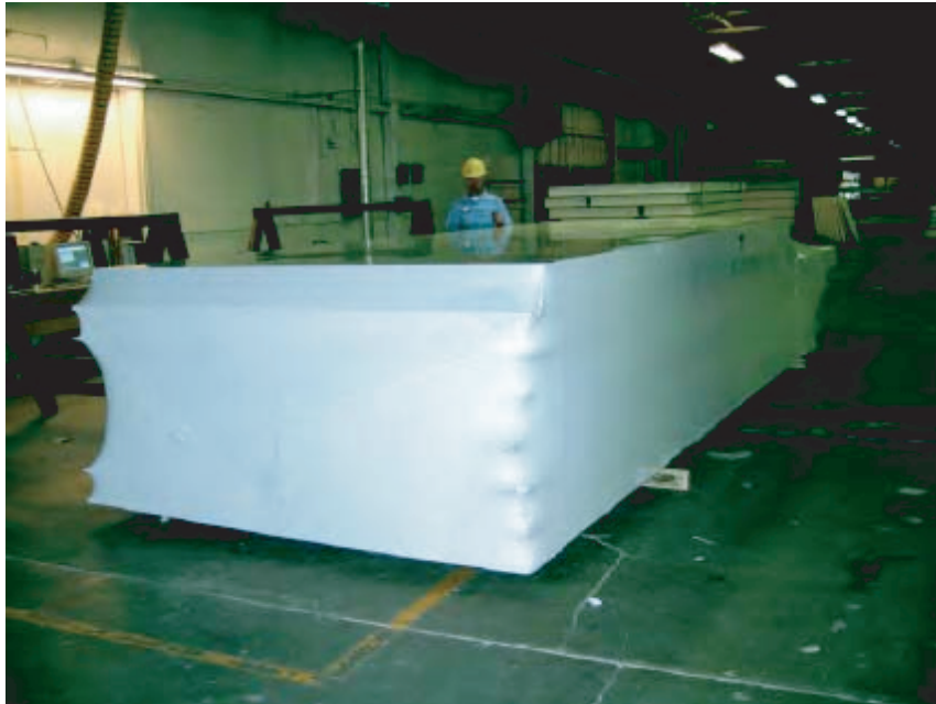
PorterSIPs are shrink wrapped at the factory for weather protection.
