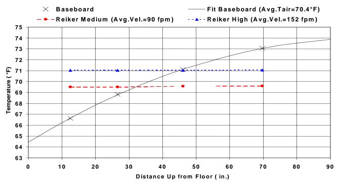
Figure 3. Stratification of Air Temperature from Floor to Ceiling of the Room from Structural Insulated Panels.
