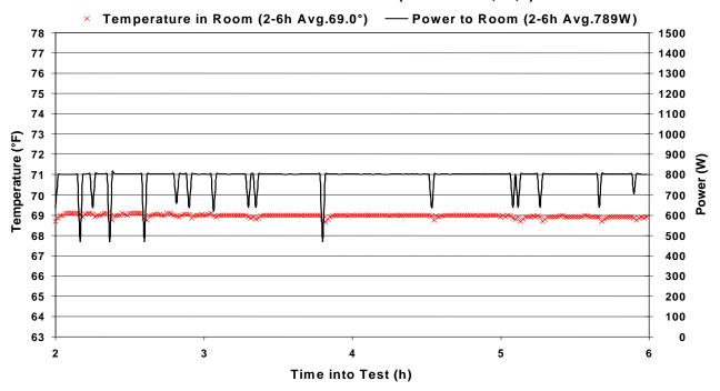
Figure 1. Example of Variation in Air Temperature and Heating Input Power for the Reiker Room Conditioner in the Room from Structural Insulated Panels.
