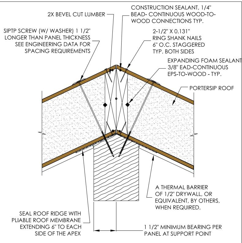
ALL FASTENERS SHOWN ARE MINIMUM REQUIREMENTS AND MAY BE CHANGED BY THE ENGINEER OF RECORD TO MEET DESIGN REQUIREMENTS.
