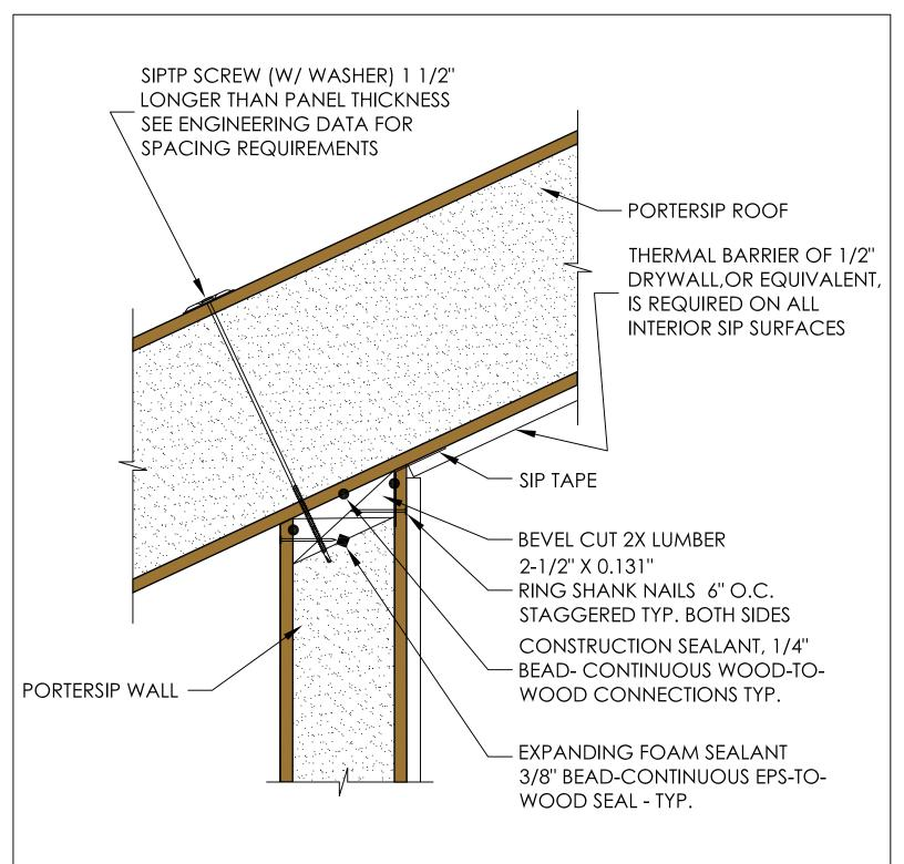
ALL FASTENERS SHOWN ARE MINIMUM REQUIREMENTS AND MAY BE CHANGED BY THE ENGINEER OF RECORD TO MEET DESIGN REQUIREMENTS.
