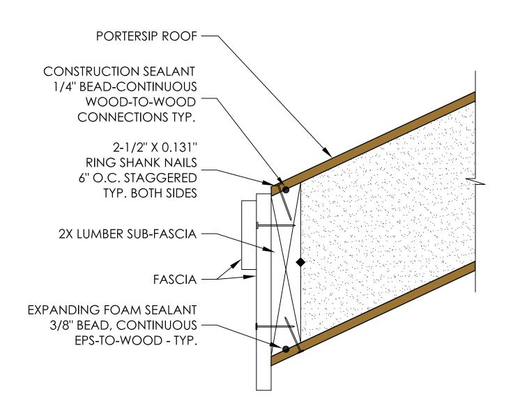
ALL FASTENERS SHOWN ARE MINIMUM REQUIREMENTS AND MAY BE CHANGED BY THE UNLESS OTHERWISE NOTED, ANY AND ALL LUMBER AND ENGINEERED LUMBER TO BE ENGINEER OF RECORD TO MEET DESIGN REQUIREMENTS.
