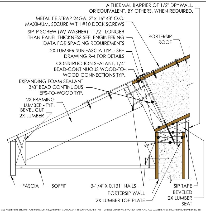
ALL FASTENERS SHOWN ARE MINIMUM REQUIREMENTS AND MAY BE CHANGED BY TH ENGINEER OF RECORD TO MEET DESIGN REQUIREMENTS. UNLESS OTHERWISE NOTED, ANY AND ALL LUMBER AND ENGINEERED LUMBER TO BE PROVIDED BY OTHERS.
