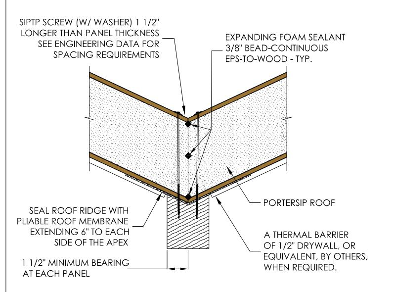
ALL FASTENERS SHOWN ARE MINIMUM REQUIREMENTS AND MAY BE CHANGED BY THE UNLESS OTHERWISE NOTED, ANY AND ALL LUMBER AND ENGINEERED LUMBER TO BE ENGINEER OF RECORD TO MEET DESIGN REQUIREMENTS.
