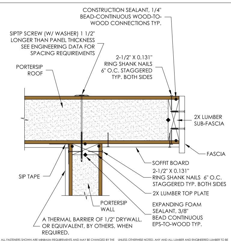
ALL FASTENERS SHOWN ARE MINIMUM REQUIREMENTS AND MAY BE CHANGED BY TH ENGINEER OF RECORD TO MEET DESIGN REQUIREMENTS.
