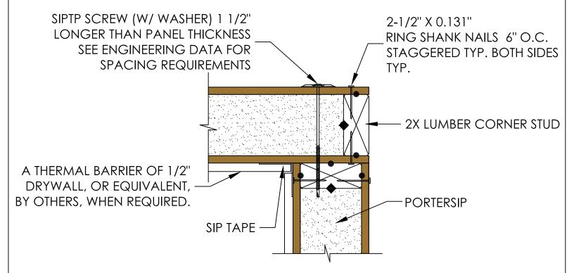
ALL FASTENERS SHOWN ARE MINIMUM REQUIREMENTS AND MAY BE CHANGED BY THE ENGINEER OF RECORD TO MEET DESIGN REQUIREMENTS.
