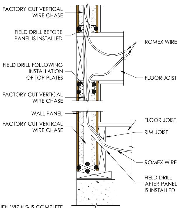
NOTE: WHEN WIRING IS COMPLETE. SEAL CHASE OPENINGS WITH EXPANDING FOAM SEALANT
